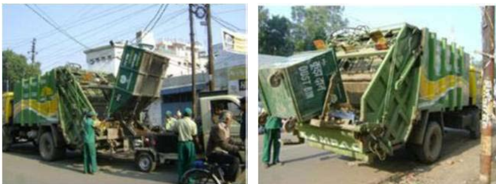
Figure 2.15: Transfer of waste from secondary collection bins to Refuse Compactor 13
