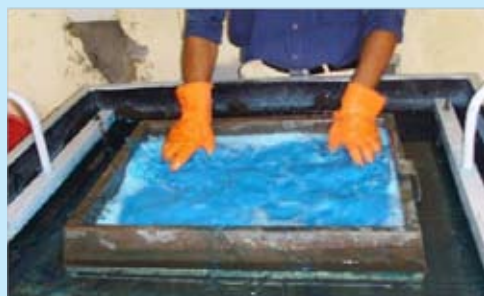
Univat being used for sheet formation
