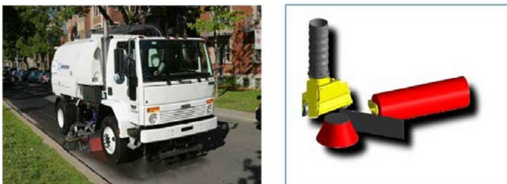
Figure 2.19: Vacuum Sweeper and Vacuum Nozzle 19
