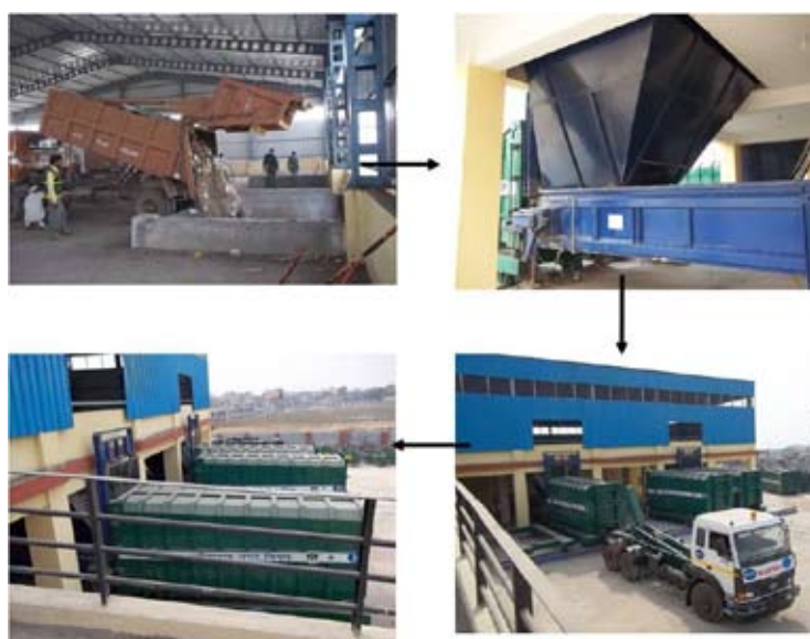
Figure 2.24: Transfer Station Operations 24
