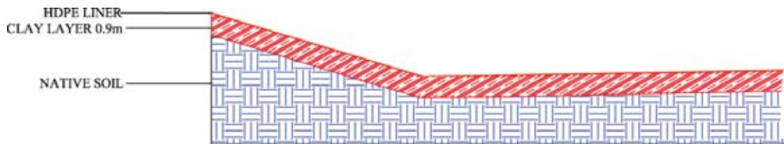
Figure 4.7: Placement of the HDPE Liner over the Clay liner
