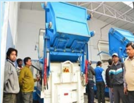
Mechanised transfer from bin to compactor
