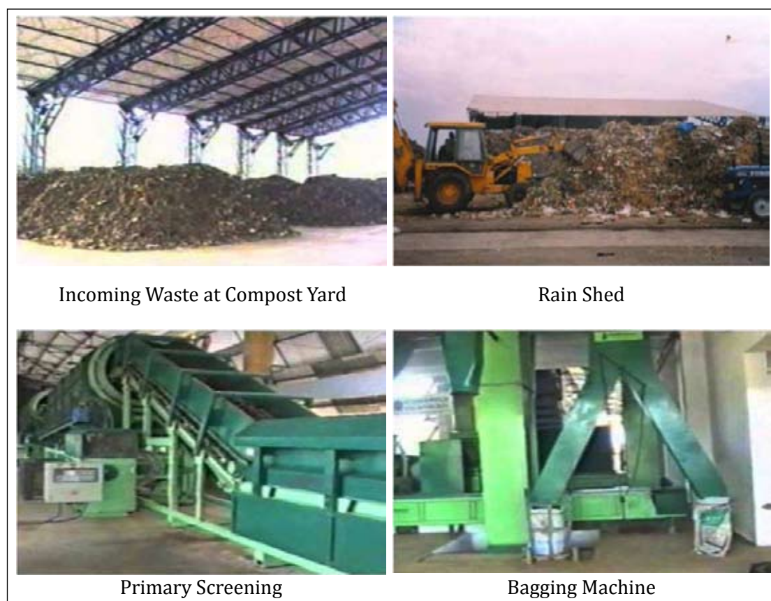
Figure 3.16: Unit operations in windrow composting
