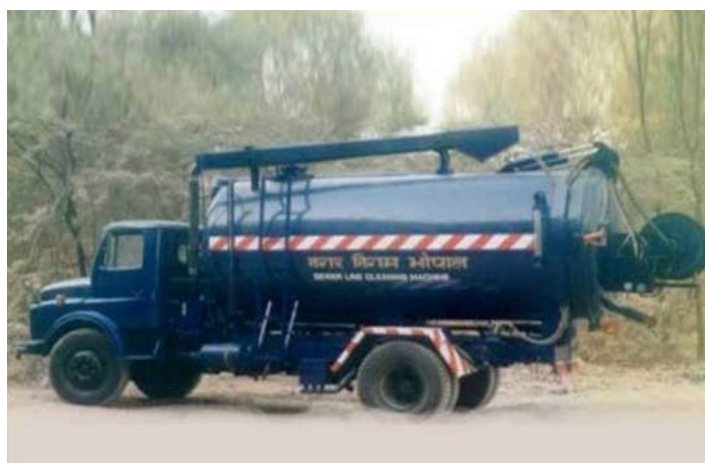
Figure 2.21: Truck mounted with pressure water jetting and suction machine 21
